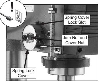
Figure 42. Feed shaft return spring assembly.
